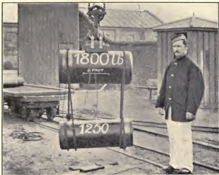
FIG. 13.—Electro-magnet for lifting heavy masses of iron. [From the "Journal" of the Institution of Electrical Engineers.]
